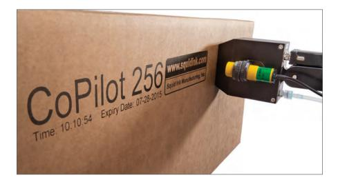
**1)** The CoPilot 256 utilizes oil-based, solvent-based, or UV curable inks for printing on a wide range of porous or non-porous substrates. **2)** A 4.3" full color touchscreen provides access to the systems internal messages and print functions.
