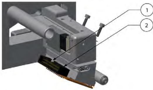
Fig. 10.5 Disconnect the cable plug from the printhead socket
