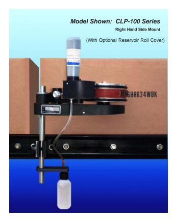
Universal's Conveyor Line Printers automatically print data on moving cartons and other flat surfaced materials with unsurpassed accuracy and legibility. These machines are mounted right on the conveyor line and require no power or operator assistance to print high quality impressions thousands of times a day.
